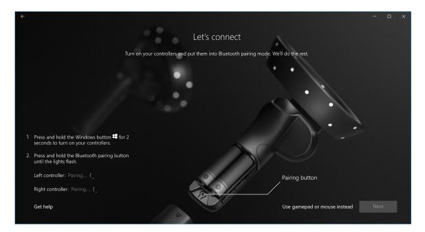
Figure 7. Pairing the visor controllers
