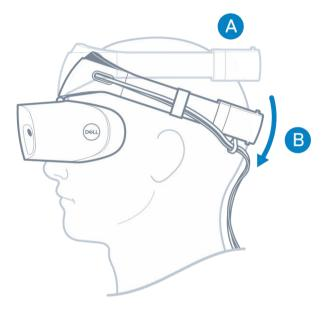
4 Use the thumbwheel at the back of the headband to obtain a proper fit (clockwise tightens the headband and anti-clockwise loosens it).
