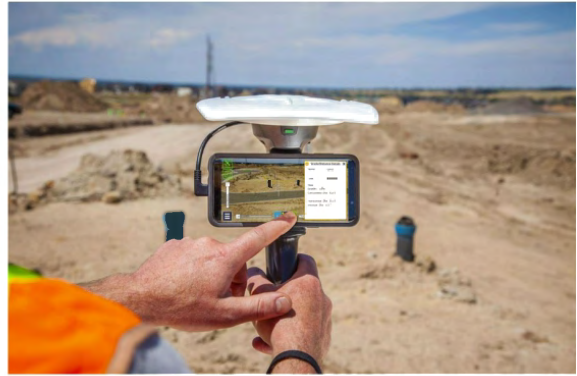
Figure 2. Handheld AR tablet device with GNSS tracking hardware.
