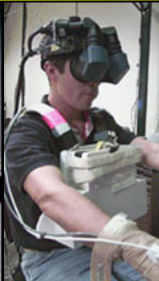
VRL Custom HMD Oculus DK2 displays - one for each eye
