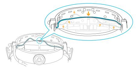
3. Reattach the front pad and side cushions to the headset band. Make sure that the side cushions cover the metal clasps on the band.
