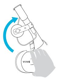
**3.** Hold the visor to your eyes. Adjust the position of the visor until you see a clear image inside the headset.
