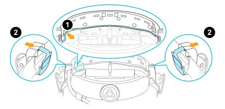
After detaching the on-ear headphones, you need to attach cable guides before plugging in your own earphones. For details, see Attaching the cable guides to the headset band on page 37.
