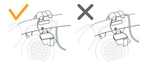
6. Close the clasp around the band and snap into place.
