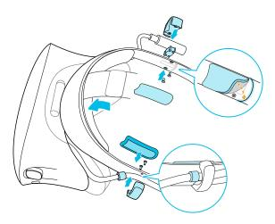
After attaching the cable guides, you can now plug in the earphones. For details, see Plugging in your earphones on page 36.
