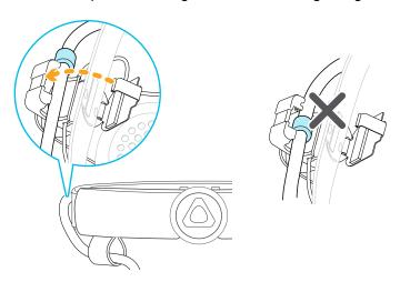
**5.** Make sure the audio cable runs under the band, and not over the top. Check that it isn't also wedged between the clip and the band.
