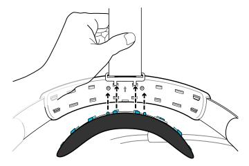
Make sure to minimize the gap between the pad and the band.
