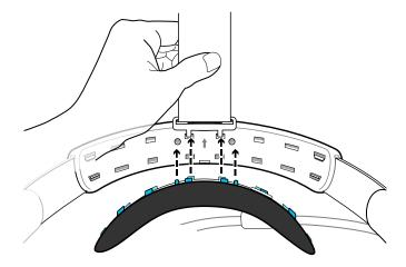
4. Make sure to minimize the gap between the pad and the band.
