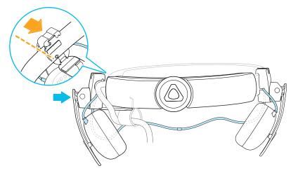
While the clasp is loose, you can reposition the headphone clip for a more comfortable fit. Make sure that the other clip is similarly placed on its side of the band.
