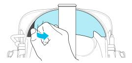
2. On the front section of the band, press the audio cable marker into the slot at the center. Then press the cable along the groove until flush with the band.
