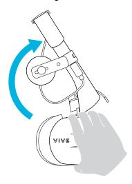
2. Detach the face cushion frame from the headset. To release the frame from its latches, gently pull on any side of the frame starting from the bottom, and then pull one side at a time on the top.
