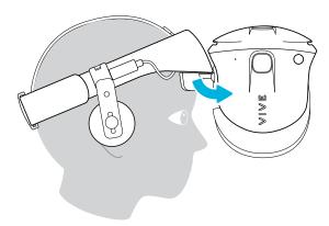
To return it to its original position, tilt the visor down until it completely covers your eyes.
