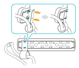
2. Reattach the top strap to the headset band. For details, see Attaching the top strap to the headset band on page 23.
