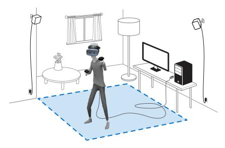
While you're in the play area, the headset and the controllers should remain at least 0.5 m (1 ft 7 in) and no further than 5 m (16 ft 4 in) away from a base station. This will ensure that the devices are properly tracked within the base station's 120-degree field of view.
