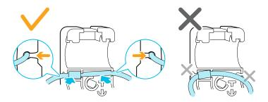
**4.** Make sure that the stopper on the headset cable isn't caught in the clasp, and is on the visor side to prevent damage to the visor while gaming.
