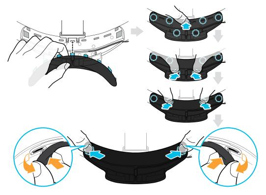
Make sure to minimize the gap between the pad and the band and that all tabs are fully locked into place.
