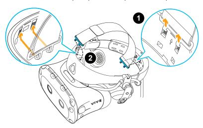
3. Reattach the front and back pads to the headset. For details, see Reattaching the front and back pads to the headset on page 18.
