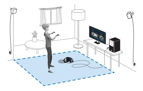
When tracing the boundaries of the play area, make sure that the floor is cleared. Do not trace across space occupied by things (such as a table or a chair) since this may cause you to trip into the object while in VR.
