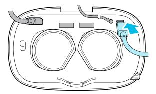
**4.** Align and push the tabs on the face cushion frame into their corresponding slots on the headset. Make sure to position the ridge of the face cushion frame below the headset, audio, and USB cables. You'll hear a click when the face cushion frame locks in place.
