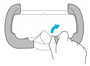
2. To reattach, align one end of the face cushion with the marker on the bottom part of the face cushion frame. Press down the face cushion against the outline of the frame, and then check that the other end of the face cushion lines up with the marker on the top part of the frame.
