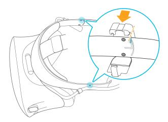
While the clasp is loose, you can reposition the headphone clip for a more comfortable fit. Just make sure that the other clip is similarly placed on its side of the band.
