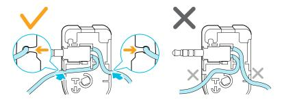
3. Make sure the audio cable runs under the band, and not over the top. Check that it isn't also wedged between the clip and the band.
