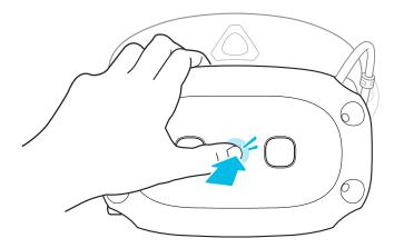
**8.** Make sure to minimize the gap between the front cover and the visor, and that all tabs are fully locked into place.
