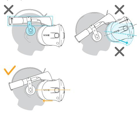
**6.** Adjust the top strap until snug, and then fasten the velcro strap.
