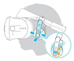
Is the fit too loose or tight? In case you feel pressure around your temples, adjust the position of the on-ear headphones for a more comfortable fit. To do so, flip open the metal clasp on each headphone and reposition the headphone clip on the headset band.
