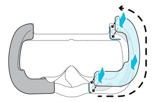
Make sure that the velcro and adhesive strips attach firmly.
