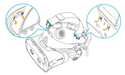
3. Reattach the front and back pads to the headset. For details, see Reattaching the front and back pads to the headset on page 18.
